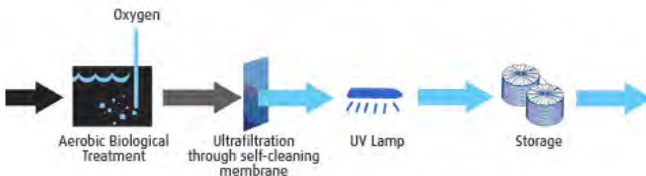
Figure 1: Water recycling filtration process.
